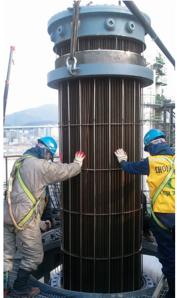
Watlow process heater bundle
