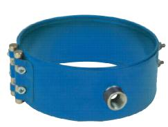
The Thermocouple Coupling facilitates the installation of an external thermocouple with a threaded fitting. The standard location for the coupling is 90° from the gap at the center of the width. Specify without through hole for heater sensing or with through hole for load sensing.
