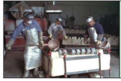
Processing aluminum castings using a Sand Mold.
