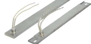
Type W1 Wire braid provides strength and protection to the lead wire insulation, offering sharp bending not possible with armor cable. 10" of wire braid over 12" long leads is standard; if longer leads or braid are required, specify.
