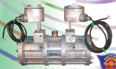
System for Pre-Heating and Mixing Chemicals for Sand Cores
