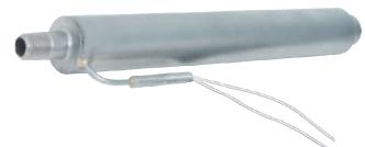
**Gas or Air Heaters** rated 1050 watts at 240 volts. One end has 1/4" MNPT and the other end has 1/4" FNPT so that you can have a series of the heaters for higher wattage requirements. It has 1-1/8" OD × 8" long stainless steel tubing body with 9-3/8" overall length.
