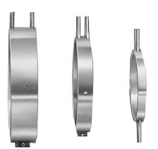
**Maxiband MXC Bands** are made for cooling only and are available in five standard widths: 3/4", 1-1/2", 2-1/2", 3", and 4". For 3/4" and 1-1/2" wide MXC bands the ends of the stainless steel cooling tubes exit 180° apart. Complete Maxiband specifications can be found on page 1-81.
