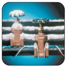
**Constant Wattage** Cable This style of heat trace cable is designed to put out a certain amount of wattage per linear foot at a particular voltage. It is always putting out the designed watts per foot, no matter what the surface or ambient temperature is. This means that in most situations the heating cable is continually pumping heat into the vessel or pipe being maintained or heat-
