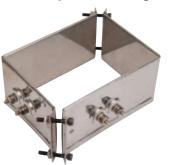
Hexagon shaped heaters are used on the hex shaped portion of the nozzle on injection molding machines. These types of heaters are strictly made to customer specifications with bent-up flange clamping only.
